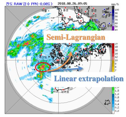
$\alpha = \tau u(t_0, x_p)$ : Linear advection  $\vec{\alpha} = \Delta t \vec{u} \left( t_0, \vec{x} - \frac{\vec{\alpha}}{2} \right)$ : Semi-Lagrangian advection  $\vec{\alpha} : \text{displacement vector,}$ - Use backward schem because of a region of a regi
