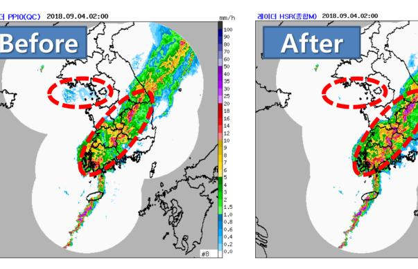
Post -processing of QPE : Raingauge Adjustment
