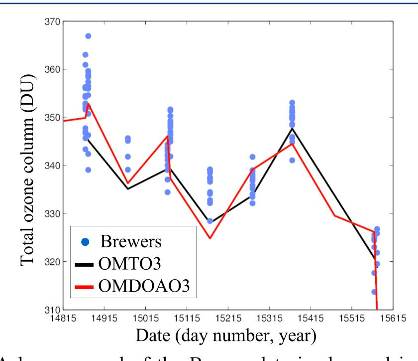
A larger spread of the Brewer data is observed in the first days of the campaign, but this should be expected, because at that point no maintenance work had been carried out. By the end of the campaign, measurements of most Brewer spectrophotometers were within ~1% of the RBCCE travelling standard.
