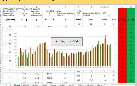
Excerpt from Badajoz balloon No.2 record. Column in red is for the value of velocity in the logbook; green column for "exact" velocity values. There are small differences but no bias has been found.
