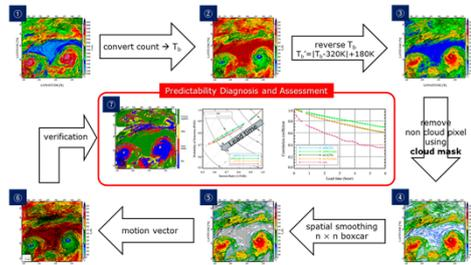
Fig. 3 Flowchart of satellite data preprocessing method based on satellite motion vector calculation.
