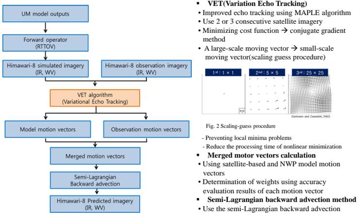
Fig. 1 Flowchart of production of the predicted satellite imagery
