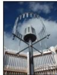
Automatic gauge (model not prescribed) with Alter shield
