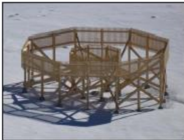
Octogonal double fence (DFIR fence)
