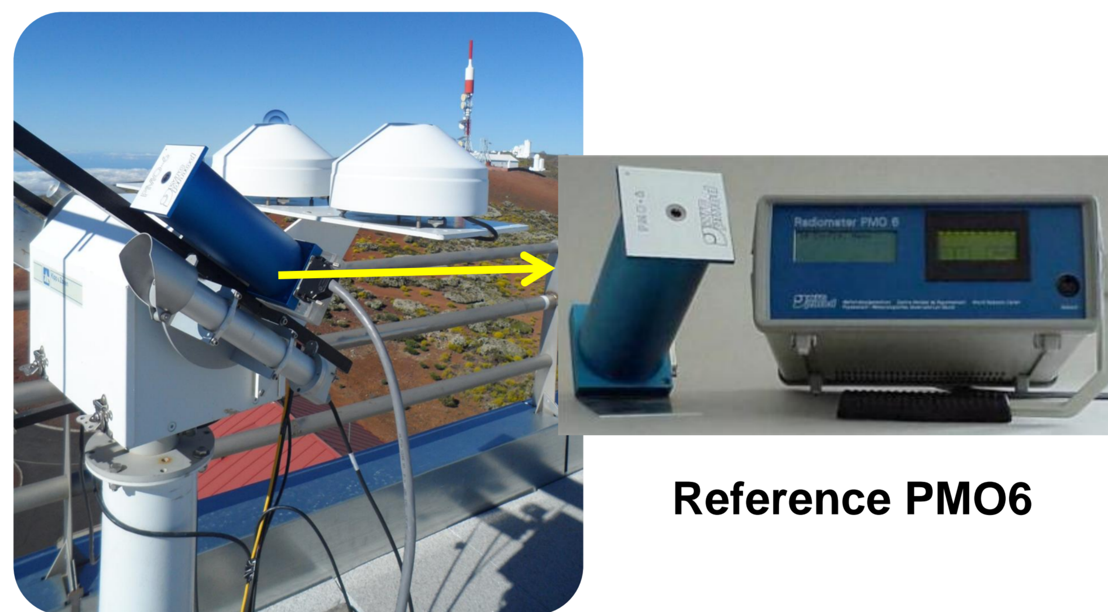
Figure 3.- Absolute Cavity Pyrheiliometer (PMO6) installed at IZA during summer 2014 in the tracker of the BSRN.
