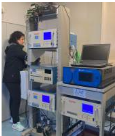
Figure 5.3. Ozone analysers (two TEI 49i and TEI 49C in the rack) at Izaña Observatory: comparison of the analysers with primary ozone standard (TEI 49i-PS)
