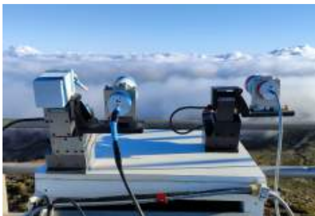
Figure 11.1. DOAS instruments outdoor optics with sky trackers and indoor set up at IZO
