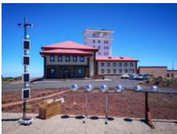
Figure 8.5. Image showing on the pole on the left, the passive mercury samplers from Environment and Climate Change Canada at the top and several PM 10 and PM 2.5 sensors below. On the right are shown the persistent organic pollutants passive samplers from CSIC.
