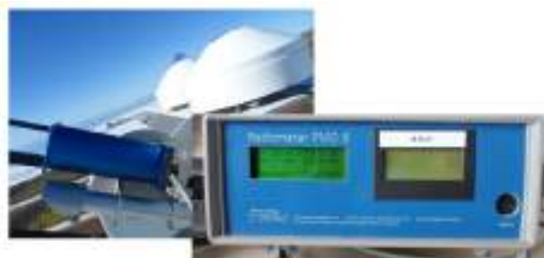
Figure 10.9. Absolute cavity radiometer (PMO6) installed at IZO during summers 2023 and 2024 on the BSRN sun-tracker
