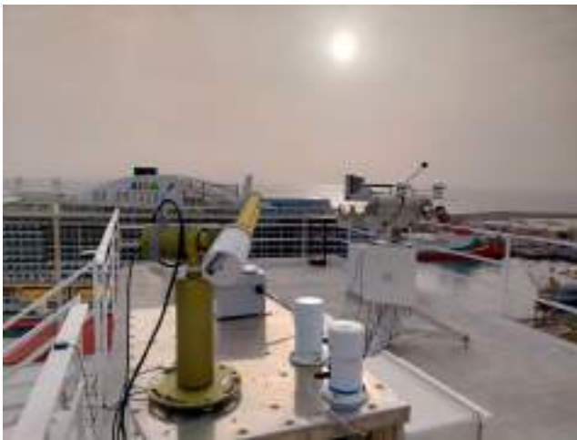
Figure 9.3. Cimel CE318-TS in operation at Santa Cruz Observatory (SCO). On the right, a ZEN, an IR radiometer, radiation instrumentation and a Hirst volumetric spore trap.
