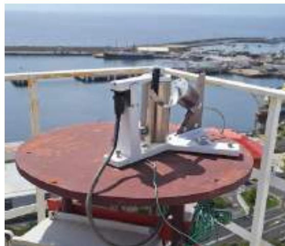
Figure 19.6. UV-MFRSR582 sunphotometer installed at Santa Cruz Observatory (Tenerife)
