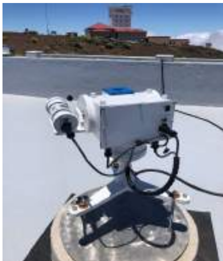
Figure 10.7. The sky scanner EKO MS 321-LR installed at IZO
