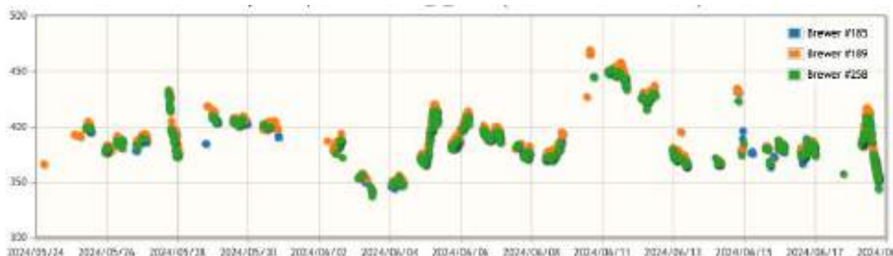
Figure 6.10. Total ozone from Brewers during CINDI-3 (24/5/2024–20/6/2024), which also included the Brewer#189, placed in the near station of DeBilt. With the calibration (provided thanks to Ankie Piters) we were able to produce V2 brewer observations which use the ozone cross section of the CINDI campaign.
