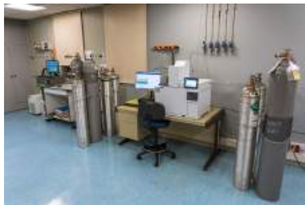
Figure 4.2. IZO Gas Chromatograph measurement system for N 2 O and SF 6
