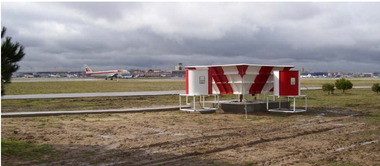
Figure 1. LAP-3000 Wind Profiler in Madrid-Barajas Airport
